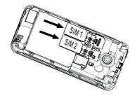
The WCDMA (SIM1) card slot supports high-speed data transmission via the "3G" mobile network. Insert here, for example, a SIM card with an Internet flat rate from your network provider.
